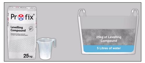
Apply Profix<sup>®</sup> Levelling Compound to **minimum** 15mm thickness for tiles or engineered wood flooring. Apply Profix<sup>®</sup> Levelling Compound to **minimum** 18mm thickness for carpet or vinyl flooring.
