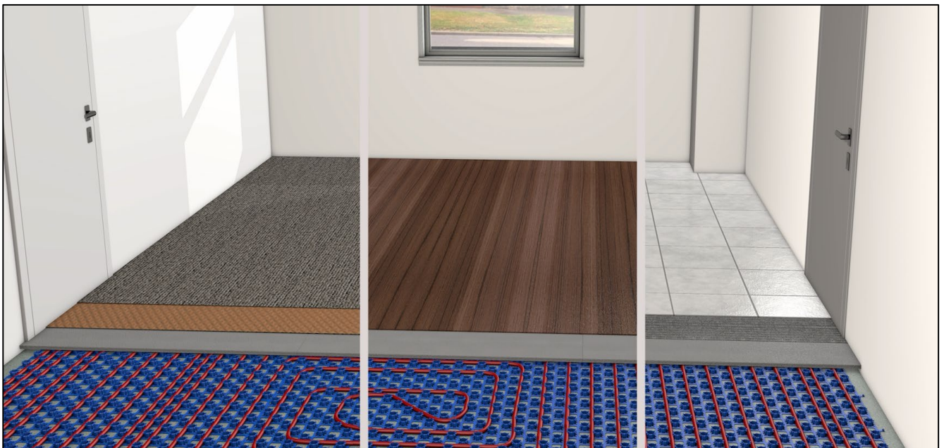
Carpet & Underlay over T & G Dry Screed Replacement Board (minimum 18mm thick)
