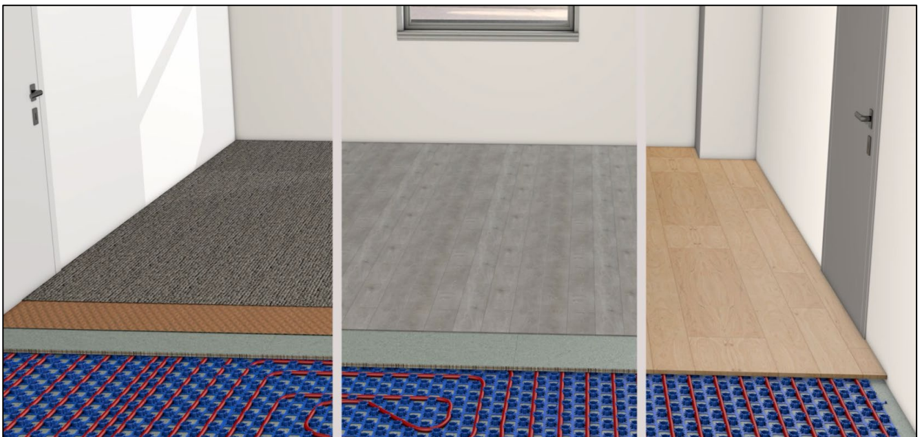
Carpet & Underlay over T & G Flooring Grade Chipboard (or similar, minimum 18mm thick)
